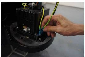
(c) Lift the column with caution and pull out all the control wires slightly.
