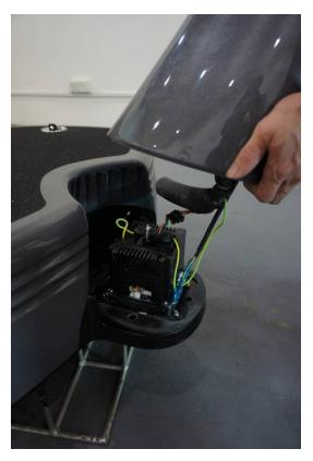
(a) Place the base plate onto the mounting rack with caution and then move the column to the wiring area of base plate.
