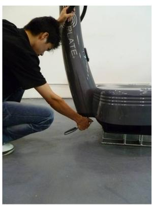
(e) Install the column with three screws, spring washers and the flat washers as shown in the picture. Make sure that the holes are aligned up and the screws are tightened properly.
