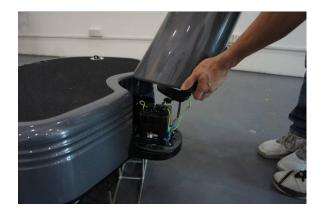
(d) Put the column onto the base plate as shown in the picture. Please be sure that the bottom holes of the column and the filter cover fit well during the assembly.
