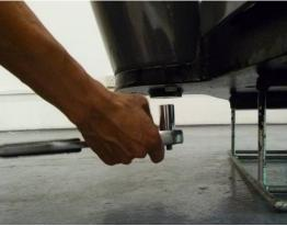
(b) Remove the three fixing screws on the column and base plate with the proper tool as shown in the picture.
